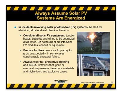
Always assume solar photovoltaic, or solar, systems are energized, whether or not the sun is shining.
