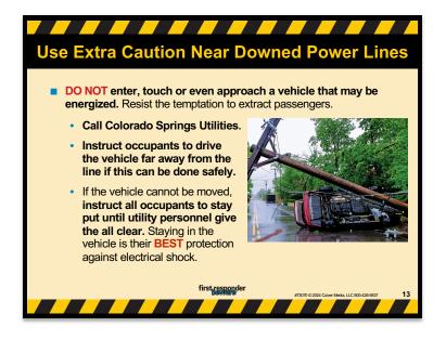
When incident victims are in or around the energized area, particularly in vehicles that have contacted power lines, remember that both you and they are safest staying put.
